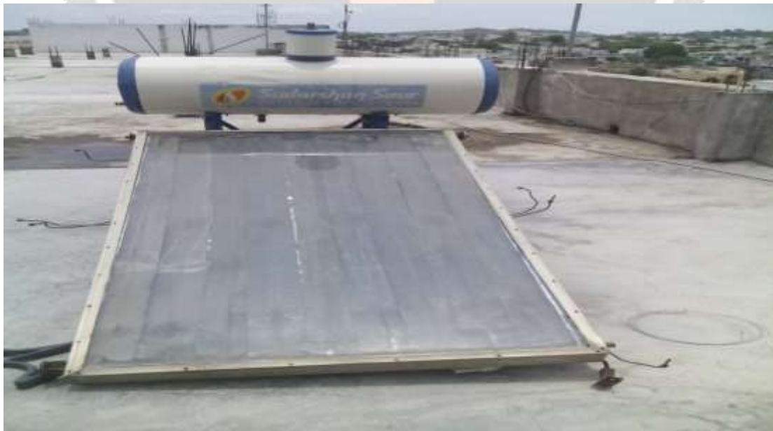
Fig.3.2 Test Rig. Of Flat plate solar water heater with insertion of twisted tape
