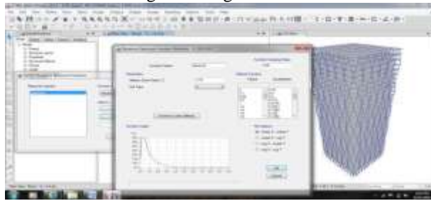
Fig.6 Defining Response spectrum data in diagrid structure
