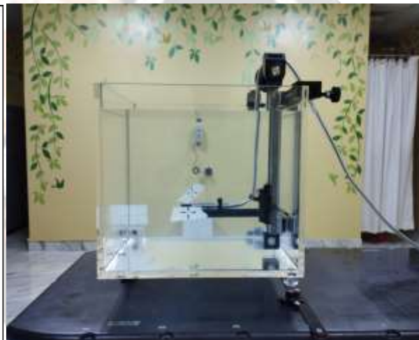
Figure -1.2: experimental set-up for the determination TPR_{20,10} and absorbed dose/MU
