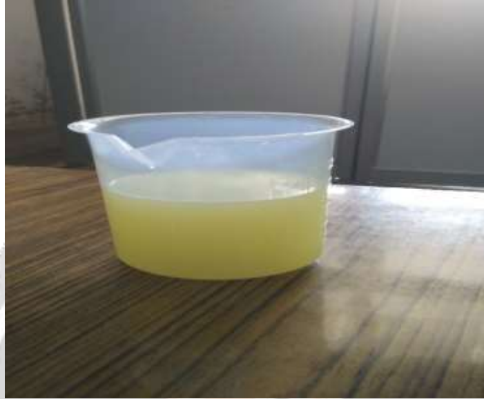
Figure 3.10 Prepared Al 2 O 3 blended Nanofuel
