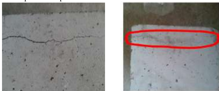
Figure .22 a) Cube with initiated crack b) Healing of crack due to B. Subtilis by M.I.C.P
