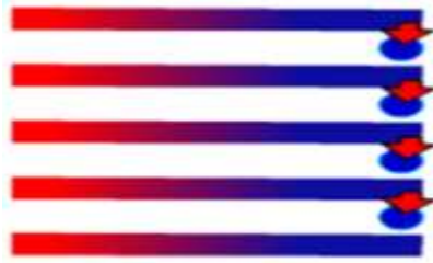
Fig.5: Cold gas takes heat from stack. Stack is colder
