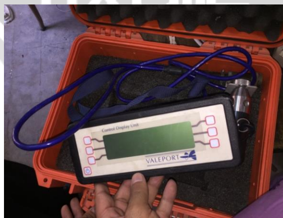
Figure (6) Employed electromagnetic flow meter
