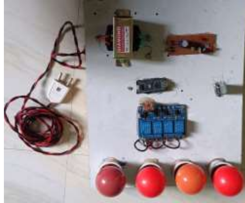
Figure5. Design of sample home automation
