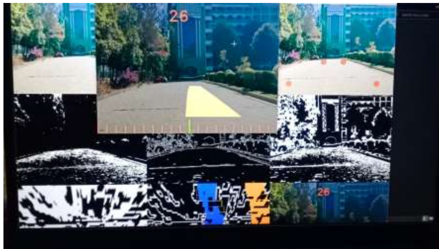
Fig -11: Value between <-50 and >60 indicates a straight path
