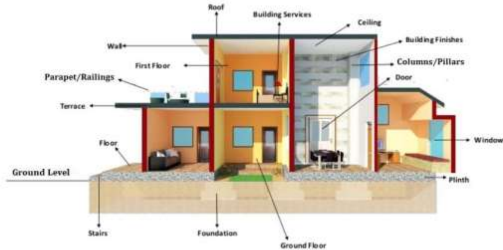
Fig.1.1. Building Basic Components : Image Courtesy: Decole
