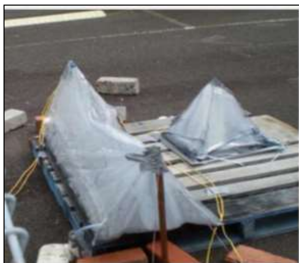
Fig.6: Long Triangular Prism Solar Still and Square Pyramid Solar Still [13]
