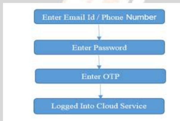
Figure 2: Existing 2-factor Authentication System for Cloud Login
