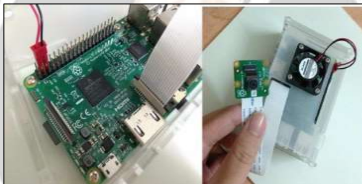
Fig. 1 Connections of pi-fan and pi-camera onto the raspberry pi 3 board with Final assembled product
