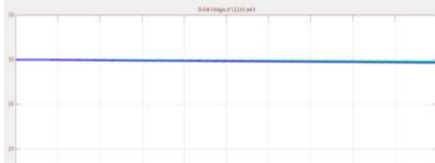
Fig-14: DC-link voltages of all six capacitors of proposed controller when using PI.
