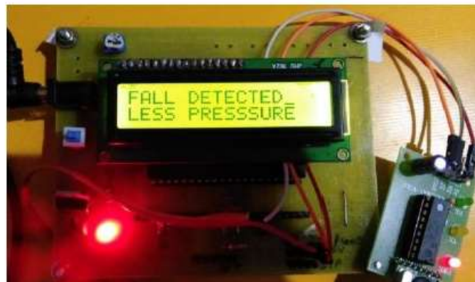
Fig: Test result of collision sensor
