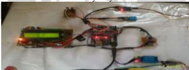
Fig.3.1 Temperature and humidity monitoring
