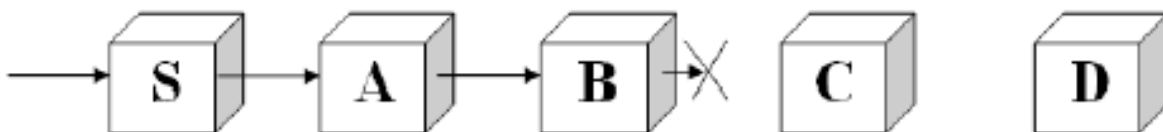
Figure 1.2: Route maintenance- node C is unable to forward a packet from S to D
