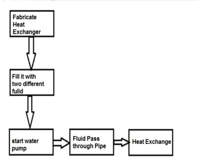
Heat exchangers with only one phase on each side can be called one-phase or single-phase heat exchangers. As we start pump water with start flowing through shell and another fluid which need to be cooled flow in to pipe, as a result heat transfer with each other.
