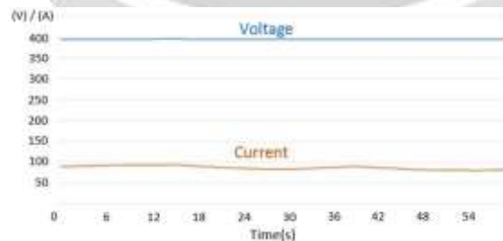
Fig. 9. Magnified view of terminal voltage, current and temperature of the tested battery set using conventional CC/CV method.
