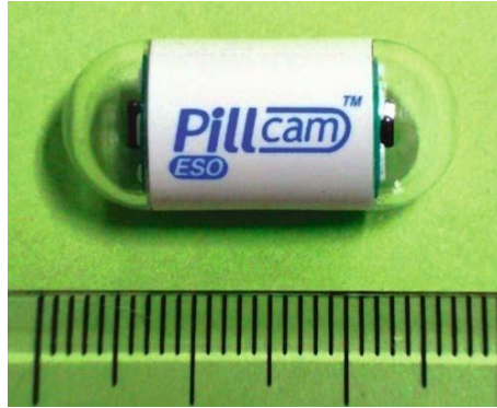
Fig. 3. PillCam ESO (11 mm x 26 mm): capsule endoscope for investigating esophageal diseases
