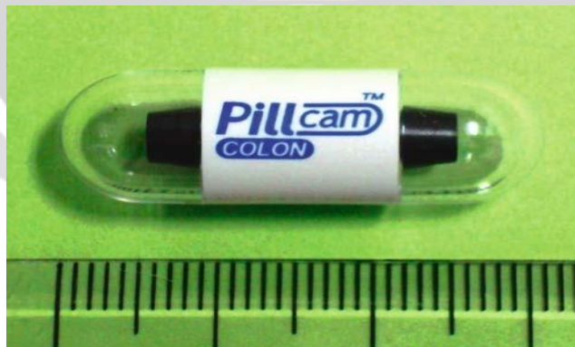
Fig. 6. PillCam COLON (11 mm x 31 mm): capsule endoscope for detecting colonic neoplasias
