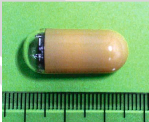
Fig. 4. PillCam SB (11 mm x 26 mm): a first-line tool for the detection of abnormalities of the small bowel
