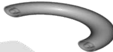
Fig 2 Close-up of double pipe coil
