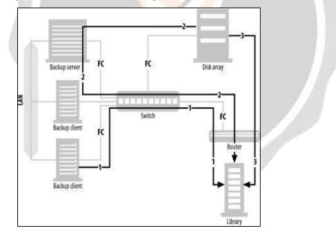
Server-free backup: The backup server; the backup client is never used to transfer data. This is known as client-free backup as a result. Client-free backups are depicted by arrow number 2, which depicts a data path from the disc array to the shared tape library after passing through the backup server, SAN switch, and router.
