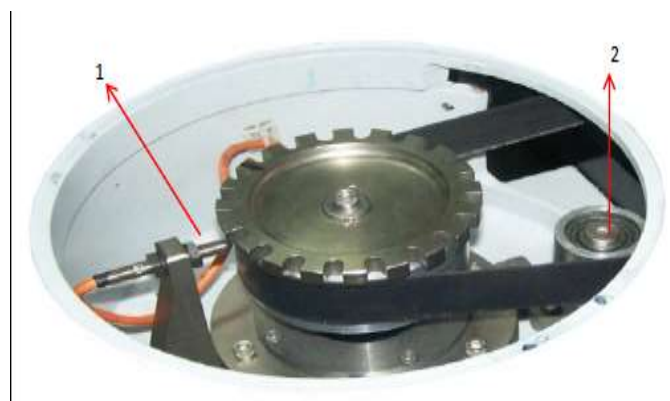
[1] Proximity sensor [2] sensor disc
