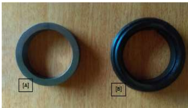
[A] Tungsten carbide seal [B] resin impregnated carbon seal
