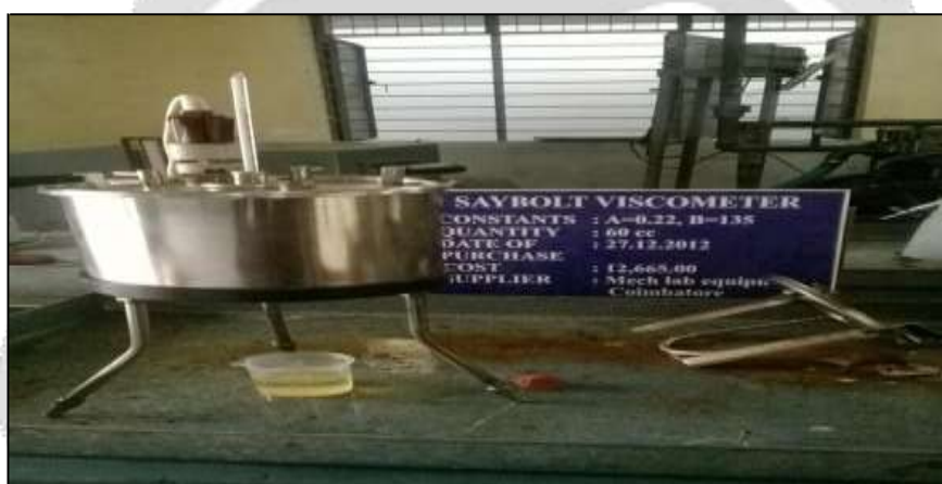
Fig 4.8 Say bolt viscometer
