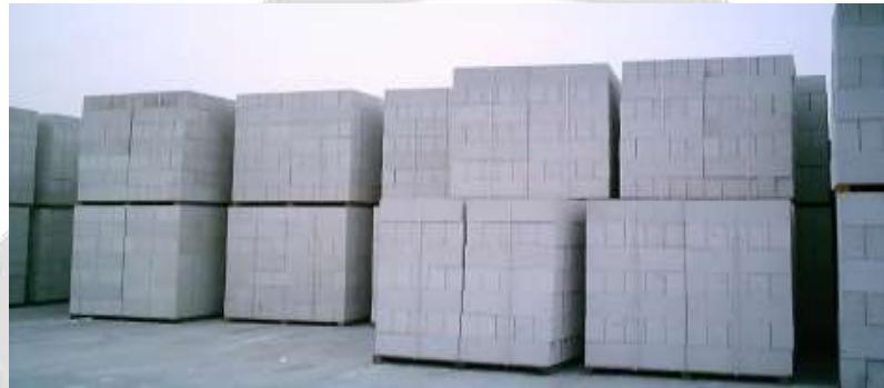
Fig -4: BLOCK FOR LOAD STRUCTURE
