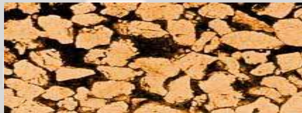
Figure 4: Oil is captured under huge pressure in pores between the rocks.
