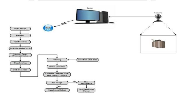
First System will take input from live video feed that is capture by any camera. This live video feed is composition of many frames. And we do the different preprocessing techniques on these frames like blurring. By applying various techniques like thresholding, Blob Detection, Filtering, Motion Detection in background subtraction technique, the desired suspicious object is detected. When the object is detected as suspicious the system will raise an alarm and send mail.
