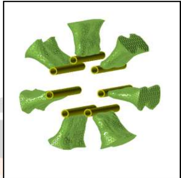
Figure -9: the topologically optimized structure of design space that have mimicked the real time structure of the wheel the wheel for 15% of maximizing the stiffness matrix
