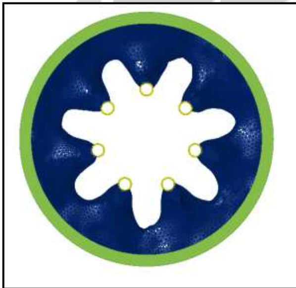
Figure -10: the topologically optimized structure of the wheel for 5% of maximizing the stiffness matrix
