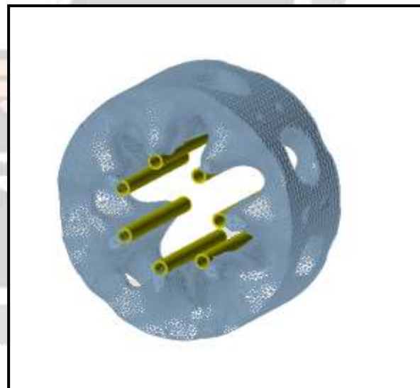
Figure -11: the topologically optimized structure of design space that have mimicked the real time structure of the wheel the wheel for 15% of maximizing the stiffness matrix
