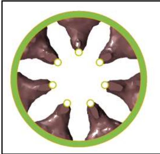
Figure -3: the topologically optimized structure of the wheel for 30% of maximizing the stiffness matrix
