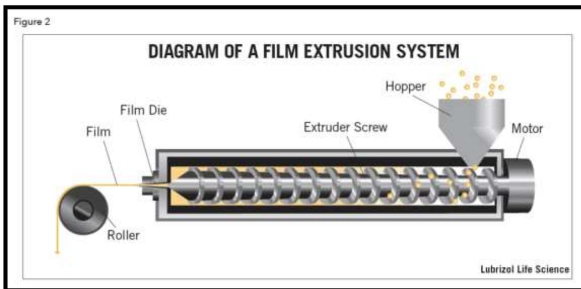
Figure 4: Hot melt extrusion technique.
