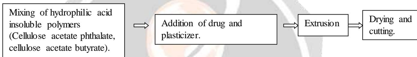
Figure 5: Flow chart of hot melt extrusion method.
