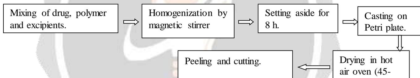
Figure 3: Flow chart of solvent casting method.
