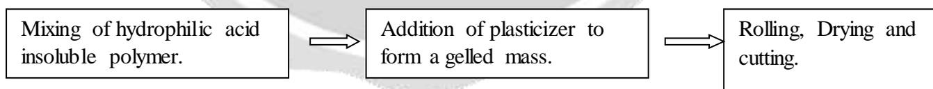
Figure 6: Flow chart of semi-solid casting method.
