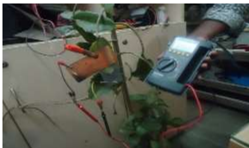
Fig.1 The measurement technique of the open circuit voltage for single pair
