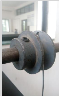
Fig -2 Rope and pulley mechanism
