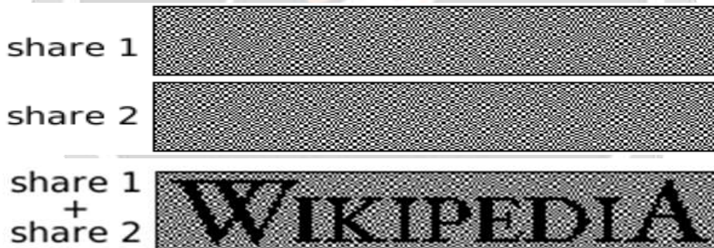
Figure 2. Visual cryptography example [15]
