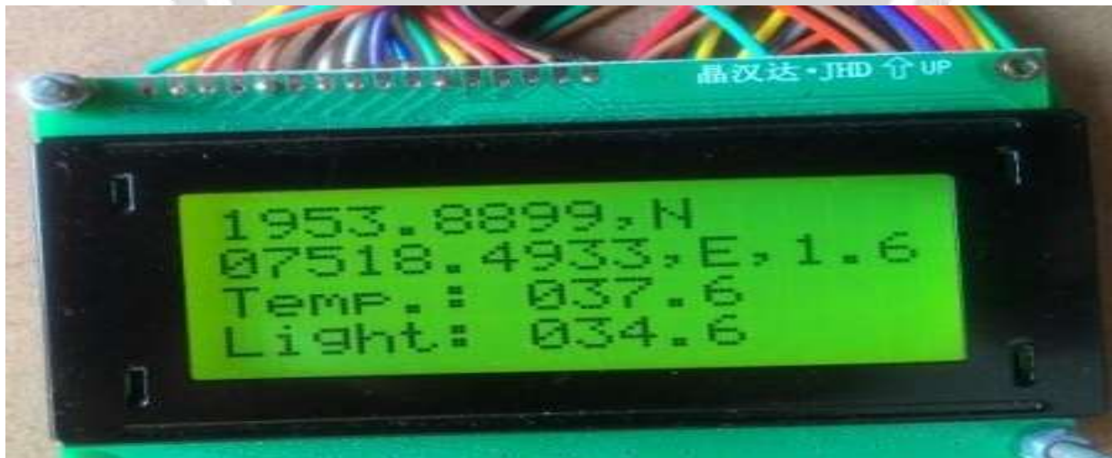
Figure 6: A part of output on Master display unit
