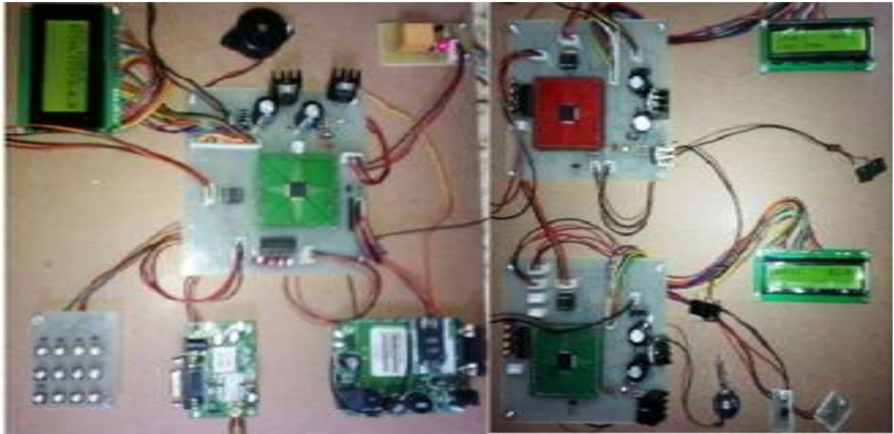
Figure 5: Actual Implemented circuit of Advanced Safety system for Vehicles using CAN
