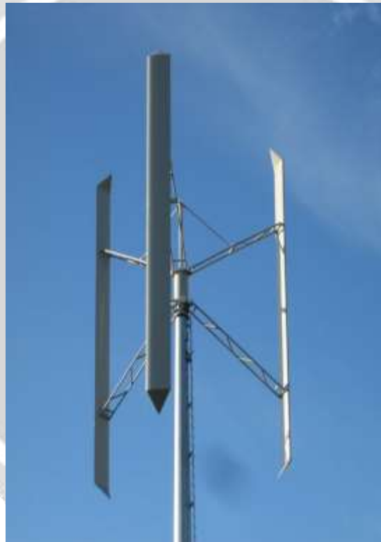
Figure No 1:- Straight Blade VAWT
