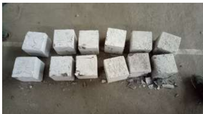
Figure 5 Failure Samples after durability attacks
