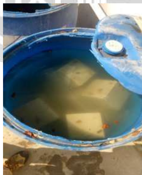
Figure 4 Cubes immersed in acid solution
