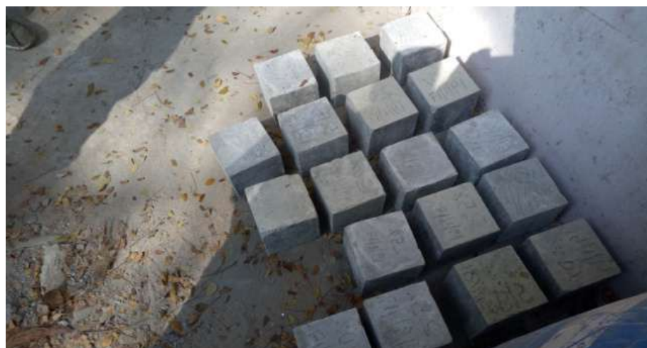
Figure 1 Cubes after 28 days of water curing
