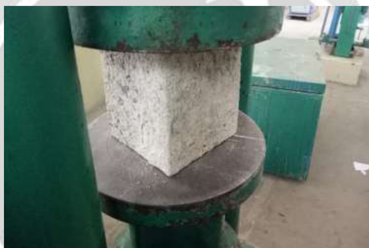
Figure 1 Cubes after 28 days of water curing
