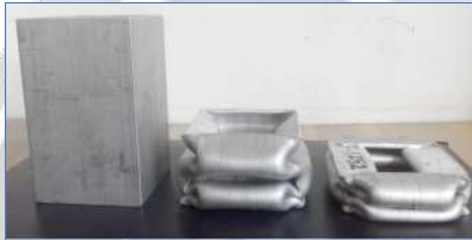
Fig -3: Undeformed and deformed crash box specimen 1 and 2
