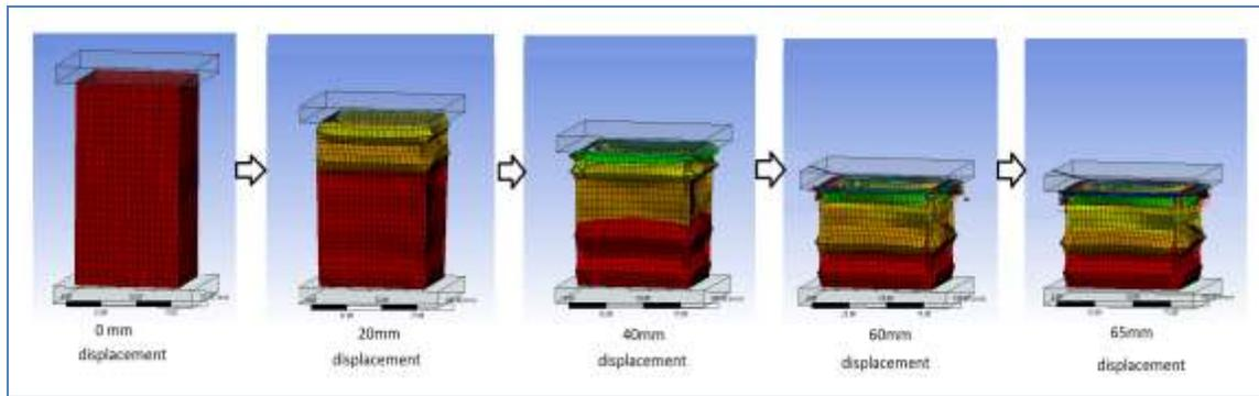
**Fig -4:** Deformation of Plane crash box.
