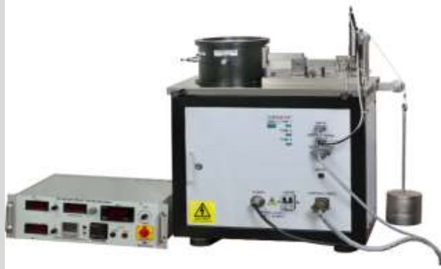
Fig. 5 Pin on disc wear test apparatus
