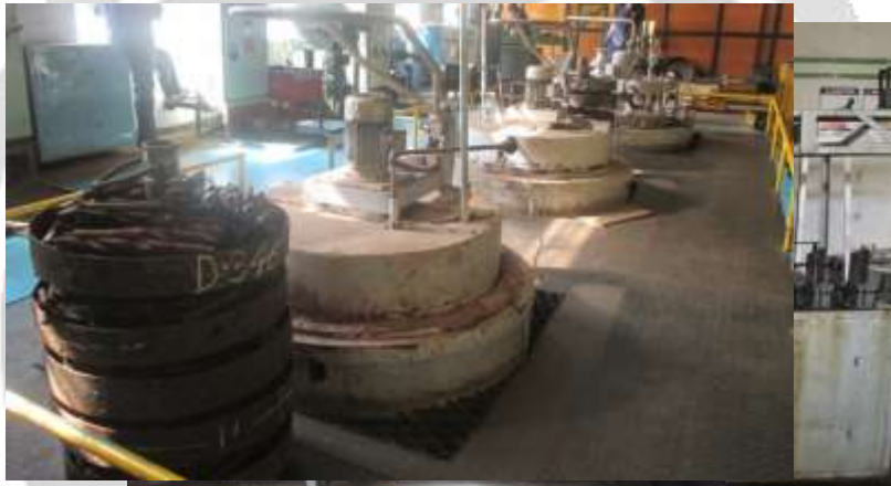
Fig2- Auto hardening setup installed at JKFIL, chiplun
