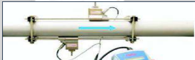
Fig -4: Ultrasonic flow meter
