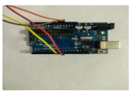
The Arduino UNO is an microcontroller board based on Microchip ATmega328P microcontroller and developed by Arduino.cc the chip is integrated with set of analog and digital input/output. The board has 14 digital pin and 6 analog pin and is programmable with Arduino IDE.
