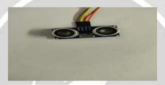
The ultra sonic sensors emits short, high-frequency sound pulse at regular intervals if strikes an object, then they emit signals that are detected by nearby system and the timespan between the emitting signal and receiving echo are used to compute the distance.
