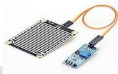
Fig -4: Rain Sensor
