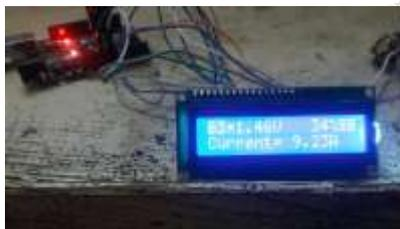
On the monitor (LCD Board) and interface display showing all real time status of all the parameters at NO - LOAD and at LOAD CONDITION – voltage, current, temperature, state of charge, state of health of every individual cells. And it's shown that our Battery management system (BMS) works perfectly.
