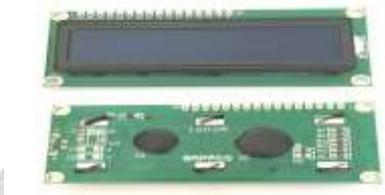
Operating Voltage is 4.7V to 5.3V. Current consumption is 1mA without backlight. Alphanumeric LCD display module, meaning can display alphabets and numbers. Consists of two rows and every row can print 16 characters. Each character is build by a 5x8 pixel box. Can work on both 8-bit and 4-bit mode. It can also display any custom generated characters Available in Green and Blue Backlight.
