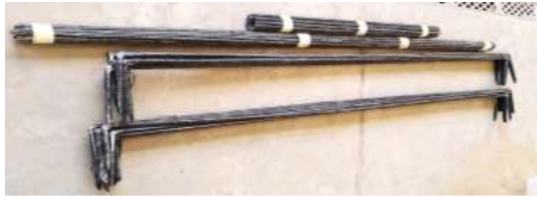
Fig.2: carbon glass fiber reinforced polymer bars (CGFRP)
