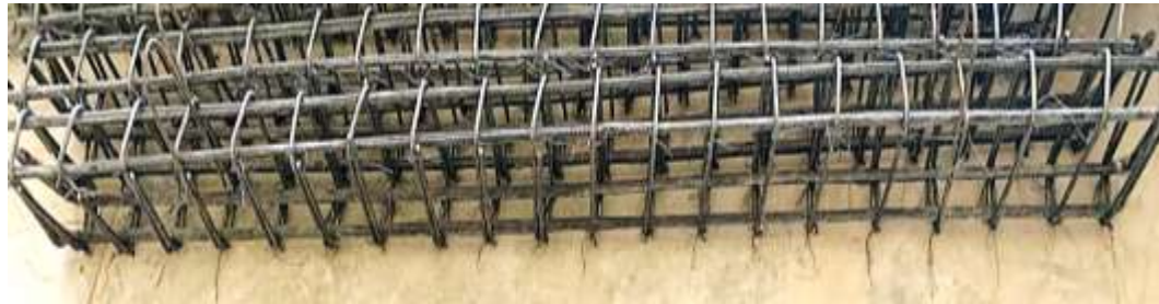
Fig.4: CGFRP reinforcement for beams
