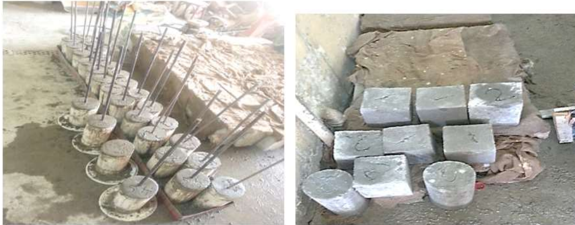
a) Pull-out test specimens' preparation b) Part of standard cubes and cylinders after curing Fig. 6: samples of the standard cubes and cylinders used in the experimental tests
