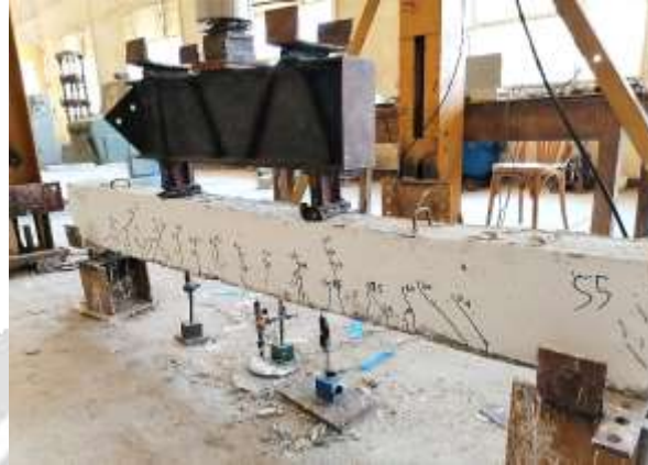
Fig. 7: Controlled four-point load compression machine.
