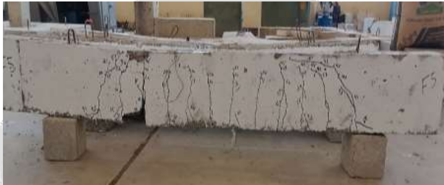
a) Reinforced with CGFRP bars.
