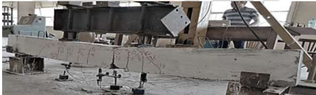
b) Reinforced with CGFRP bars
