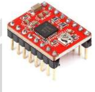
Fig -10: A4988 Stepper Motor Driver
