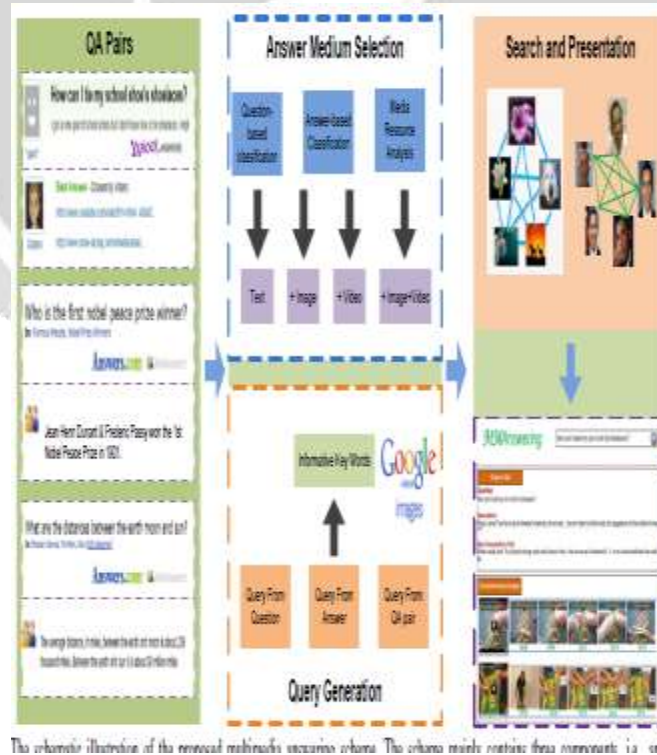
Fig 2. The schematic illustration of the proposed multimedia answering scheme. The scheme mainly contains three components, i.e., answer medium selection, query generation, and data selection and presentation.
