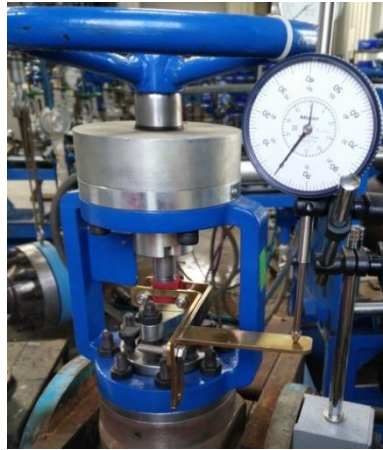
Fig 4: Dial gauge arrangement for lifting stem
