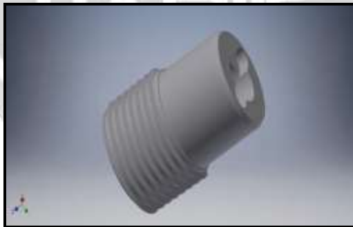
Fig.-6: Flow Control Valves (FCV) Part3
