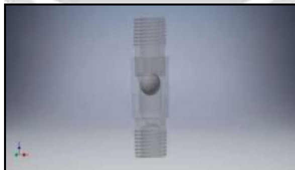
Fig.-9: Transparent Flow Control Valves (FCV) Re-assembly
