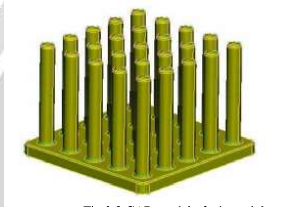
Fig.2.2 CAD model of a heat sink
