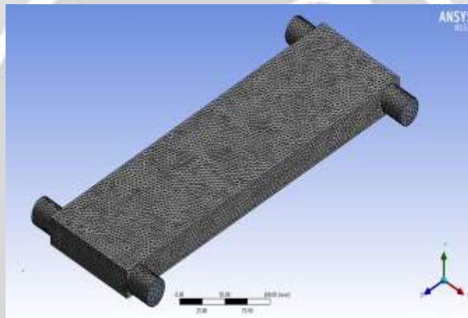
Fig. 3: Mesh diagram of mini channel heat exchanger
