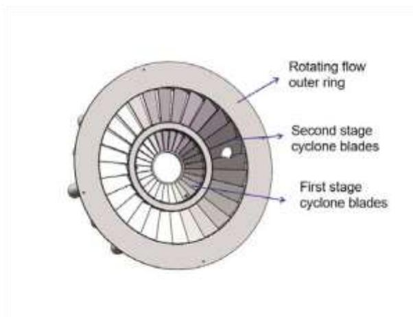
**Figure 3.** Structure of a flame holder
