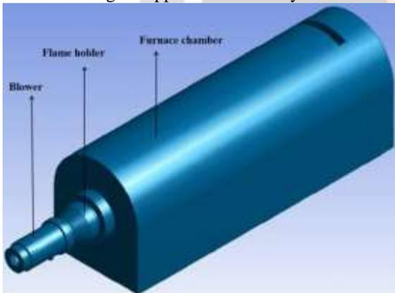
**Figure 1.** Three-dimensional diagram of the gas heat element
