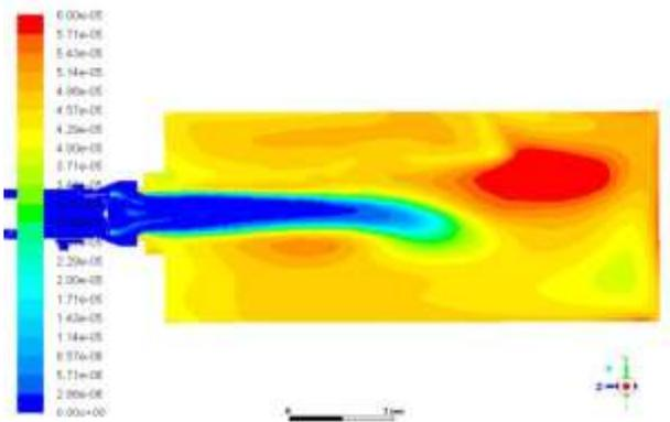
**Figure 12.** NO sequence of cross sections in X=0
