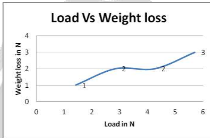
Figure 4.5: Effect of load in weight loss when tested in abrasive grit paper 4/0
