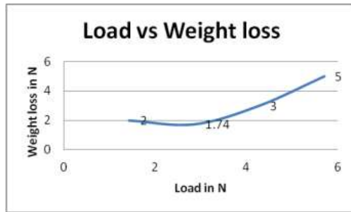
Figure 4.4: Effect of load in weight loss when tested in abrasive grit paper 3/0
