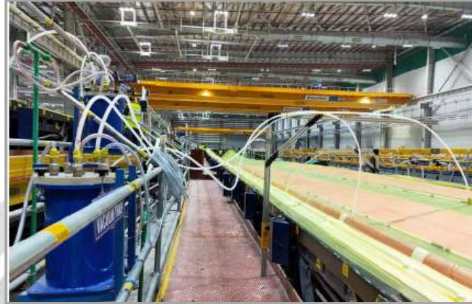
Fig 4.2 Infusion process in main mold
